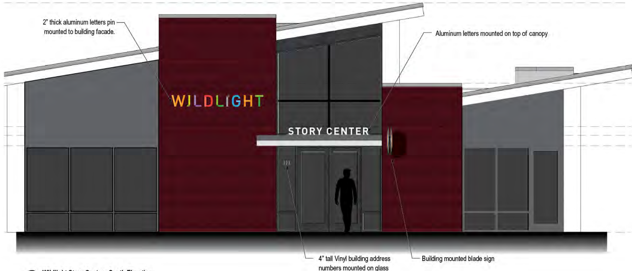
1 Wildlight Story Center - South Elevation Scale: 3/16"=1'-0"
