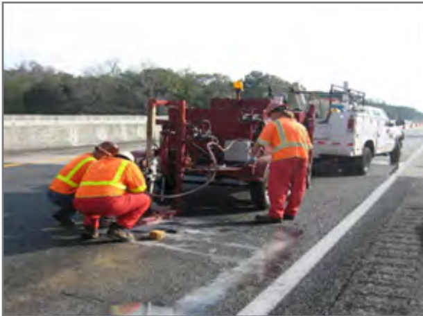
Figure 2: Photo of Standard Penetration Testing (SPT)
