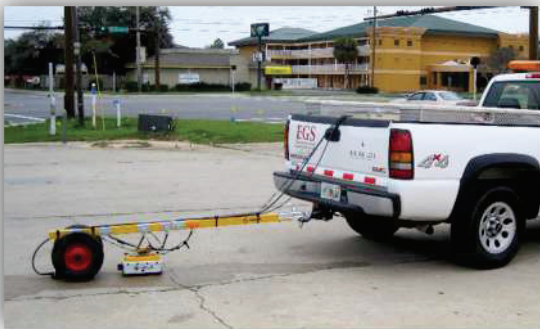
800 MHz GPR Antenna on Road Trailer
