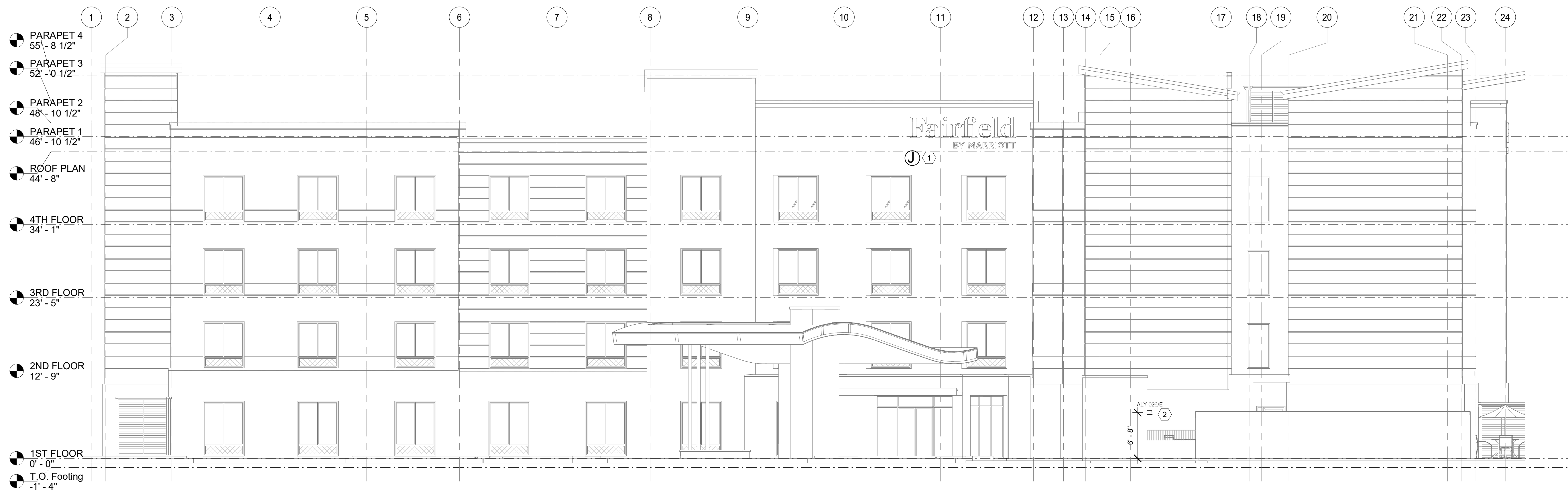
1 BUILDING FRONT ELEVATION LT-205/ 1/8" = 1'-0"
